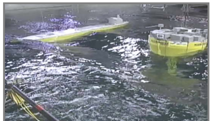
Figure 7. SSP VERSUS TRADITIONAL SHIP-SHAPED FPSO RESPONSE UNDER 100-YEAR GULF OF MEXICO HURRICANE WAVES [Ref 4]
