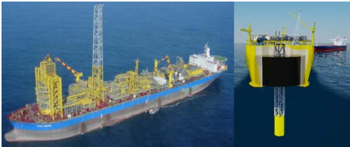
Figure 1. A TYPICAL SHIP-SHAPED AND ROUND-SHAPED FPSO
